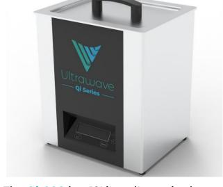
The Qi-200 is a 12Litre ultrasonic cleaner with a menu driven, LCD control panel. This allows simple adjustment of cycle time (0 to 99mins or infinity mode), temperature (ambient to 80°C), ultrasonic power and frequency mode for precise and accurate processing.
